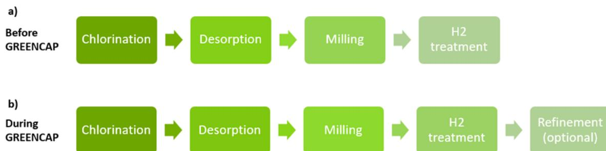
Figure 2-12 a) Curved graphene production process steps before the GREENCAP project, b) Curved graphene production processes steps during the GREENCAP project where additional refinement step is considered.
