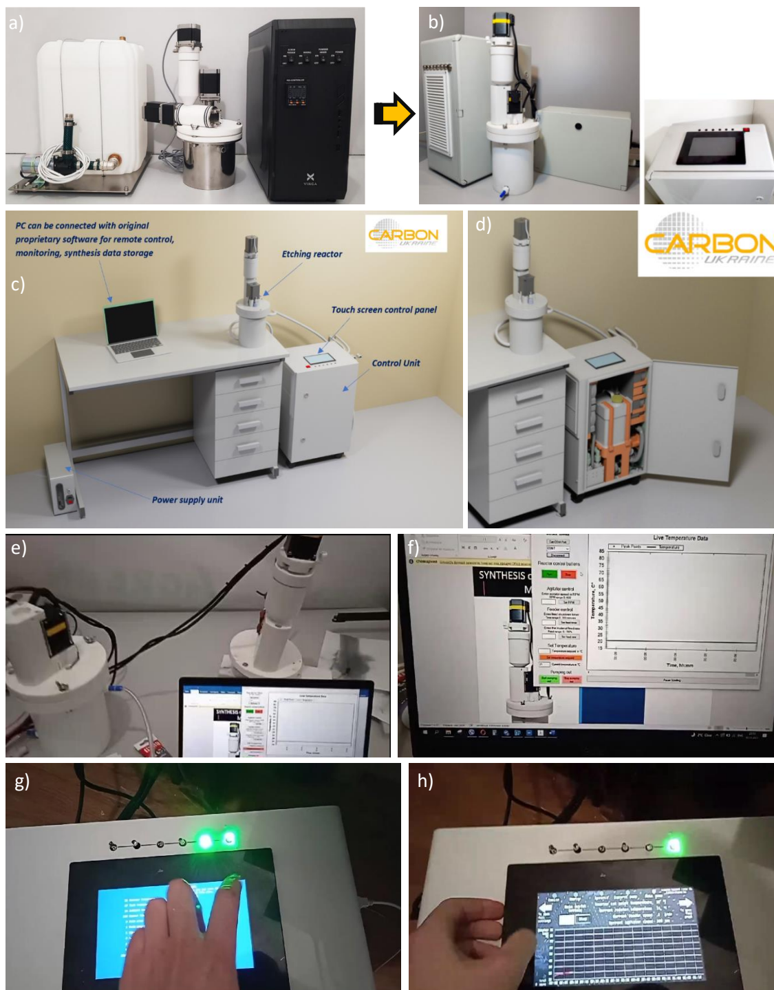
Figure 8: a) Modified Laboratory etching reactor with control system and proprietary software developed by CU; b) Previous generation of Etching reactor system; c) Complete view of the system developed by CU; d) Control unit of the etching reaction system; e,f) Interface of the control system at the connected PC; g,h) Touch screen display of the control unit.
