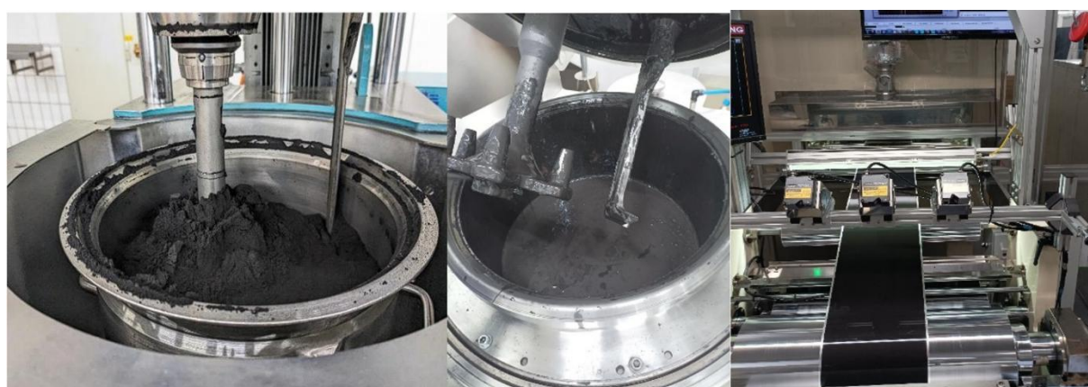
Figure 6. Mixing (left and middle panel) and coating (right panel) of electrode slurries.
